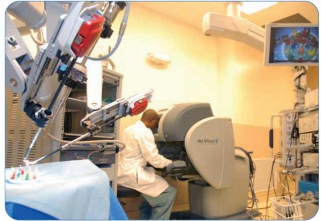
Walter Quiller, RN, Endoscopy Coordinator, tries his hand at surgery using the da Vinci robot. By using the robot arms, he can manipulate the colored objects on the operating table at the lower left. His every action can be seen on the flat screen in the upper right corner.
